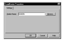
In [Station Name] enter the name of the computer on which the ScanRouter Station is running, and click the [OK] button.
